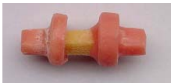
Figure 2. The specimen of cancellous bone of the femoral condyle embedded with PMMA for torsional testing
