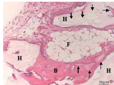
Fig. 3. Photomicrographs of HE sections at 4 weeks after the implantation of rh BMP-2/fg-HAp ceramics. B: bone, H: HAp containing body fluid, F: fatty marrow, : fragmented HAp, : osteoinduction with bone remodeling. HAp fragmented by body fluid permeation and new bone formation from surface and bulk regions of the ceramics were observed, while HAp incorporated by the induced bone with fatty marrow were found.
